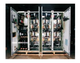
Banyard has a wide range of medium and high frequency inverters to address a comprehensive range of applications. For the heating of large diameter billets, Banyard's latest generation of IGBT low frequency inverters provide greater operating efficiency and significantly faster heating rates.
