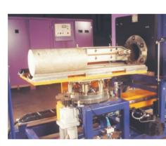
For copper and brass the rapid heating rates achievable by induction also reduce oxide formation and surface burnout of alloying elements ensuring improved product quality. Reduced grain growth and precipitation of Mg2Si in aluminium alloys improves product quality and anodising finish.
