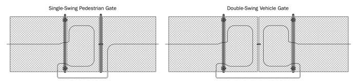
UniZone's rugged, flexible MicroPoint™ cable can be easily mounted to protect swing gates, and will withstand ongoing repetitive gate openings/closures. To prevent nuisance alarms, sections of cable may be easily disabled in software at driveways or pedestrian walkways and routed underground, without a need for splicing non-sensitive cable.
