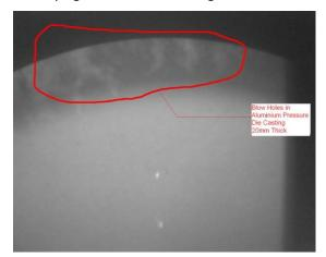
traditionally been done using sampling methods and Third Party X-Ray Inspection. This takes as lot of time and is costly. This increases the inventory and reduces the defect prevention capability of Aluminium Casting Companies.
