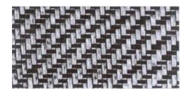
Hybrid fabric of carbon and aramid fibers Exhibit - 1c
