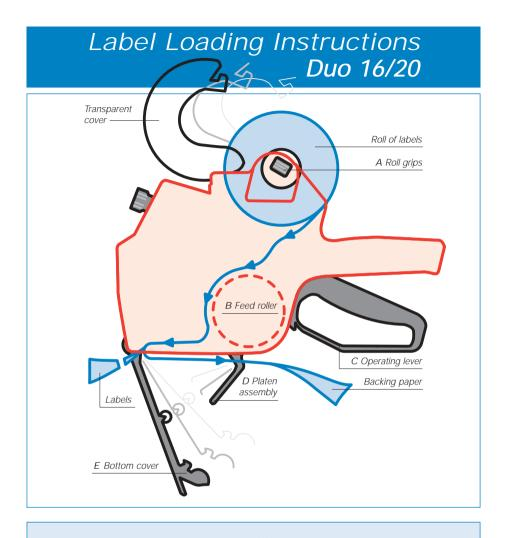
Lift transparent cover and squeeze roll grips (A) allowing roll of labels to be placed into the machine.
