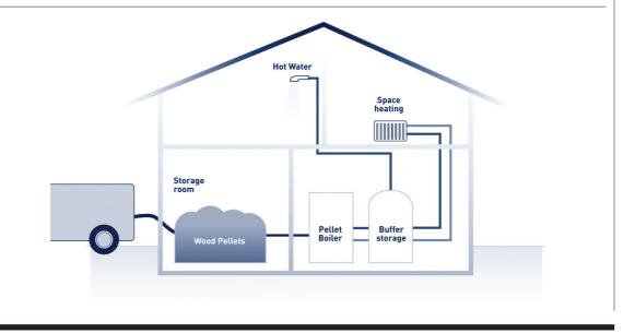
heat source like a gas boiler. For example: if the accumulator tank is too large for periods of low demand (like in summer), the gas boiler is likely to short cycle with not enough demand on the biomass boiler and the turndown ratios of biomass boilers are not as low as gas. Short Cycling is where a boiler is cutting in and out in short periods of time, this is less efficient than longer loading period due to firing up. It also increases maintenance and reducing the life time of the boiler.
