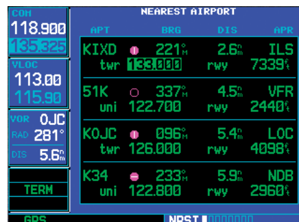
Nearest Airport Page with common traffic advisory frequency (CTAF) for the closest airport highlighted.
