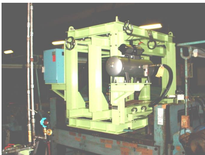
Figure 2. Experimental equipment of spot welding machine
