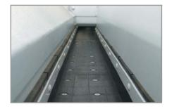
The sand and aggregate hoppers have a 4-inch vertical trough at the base ensuring accurate quantities throughout the load.
