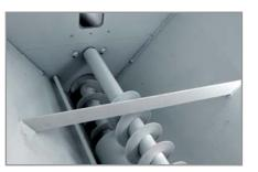
The cement hopper has twin, self-cleaning dispensing augers, meaning our machines easily conform to the stringent requirements of EN206-1 and have acheived third-party quality assurance.
