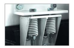
The body and cement bin are separately mounted on sprung bolts, protecting them from distortion and preventing cracks.
