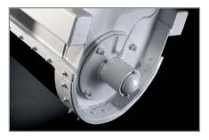
The Armcon Cementech Max-Life<sup>™</sup> auger bearing is a sealed unit, which not only extends service life by preventing slurry ingress but does away with the need for daily lubrication.
