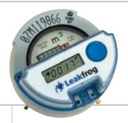
The function of the Leakfrog is to detect, store and display the maximum time between successive pulses from pulsed output meters. The maximum time between pulses is the reciprocal of minimum observable flow. The higher the value displayed on the Leakfrog, the smaller the leak.
