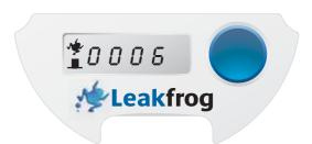
The value displayed is "0021" indicating a maximum interval between pulses of 21 seconds since the unit was deployed. Assuming the meter is calibrated to 1 litre per pulse, a value of "0021" means that a litre of water is passing through the meter every 21 seconds. This equates to a minimum flow rate of approx 3 litres per minute which indicates a leak.
