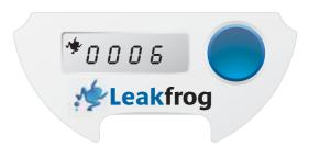
When the sensor on the meter passes directly under the sensor of the Leakfrog, a switch shaped icon " \_\_\_\_" appears on the bottom left of the Leakfrog display. This is additional confirmation of operation and will only be seen by the operator if there is high flow when they are on site, or if the unit is placed directly over the sensor.
