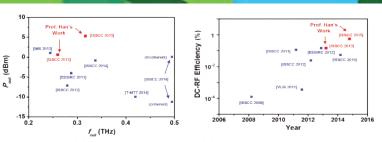
**Figure 2**. (a) The output power and (b) DC-to-RF efficiencies of the state-of-the-art terahertz radiators based on silicon integrated circuits.
