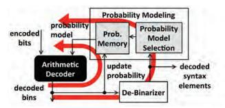
Figure 2:Feedback loops in CABAC entropy decoding engine.
