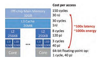
**Figure 1**: Current chips with few cores use hardware-managed hierarchies to reduce the cost of memory accesses. This figure shows the sizes, latency per access, and energy per access of an 8-core Intel E5-2670 chip running at 2.6 GHz.
