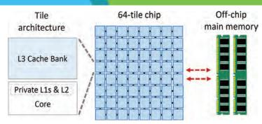
Figure 2: A tiled 64-core chip with a distributed cache hierarchy.
