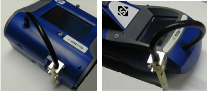
Figure 2-8: Installing Door-Oliver Cyclone
