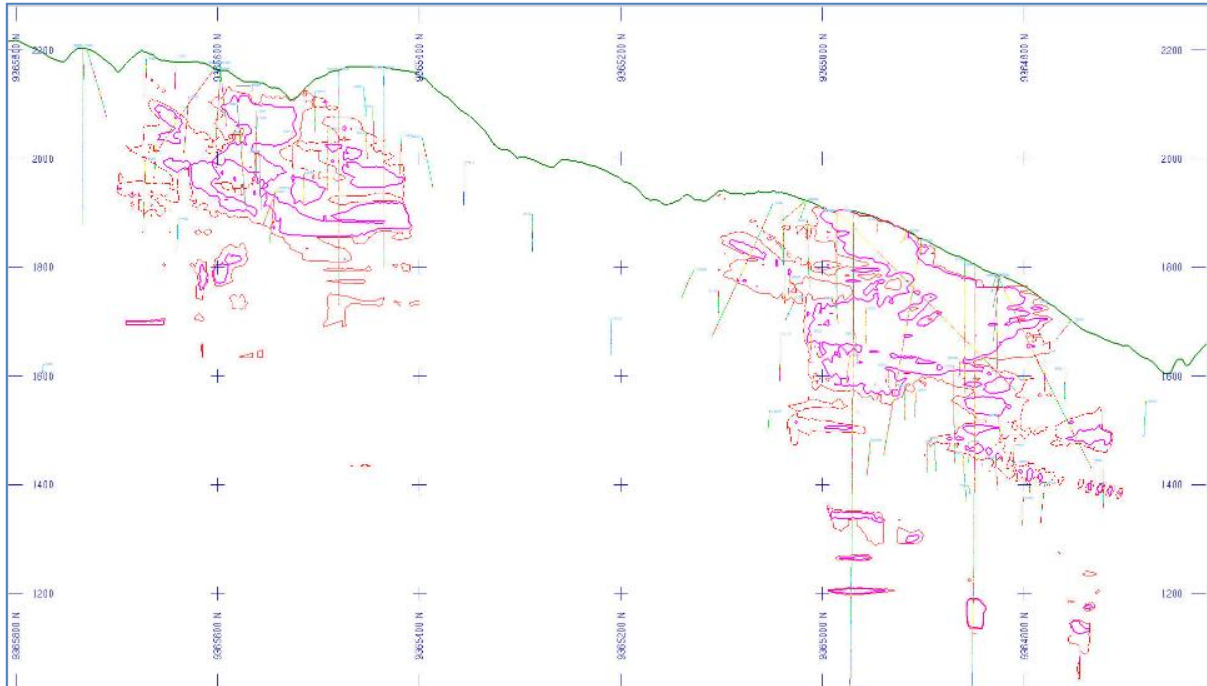
Figure 35 Yandera Long Section Schematic derived from Block Model Grade Shell Contours Depicting +0.4% (red) and +0.5% (magenta) Cu Mineralisation contours in conjunction with surface topography profile - as at 12 April 2012 (view direction approximately North-East)
