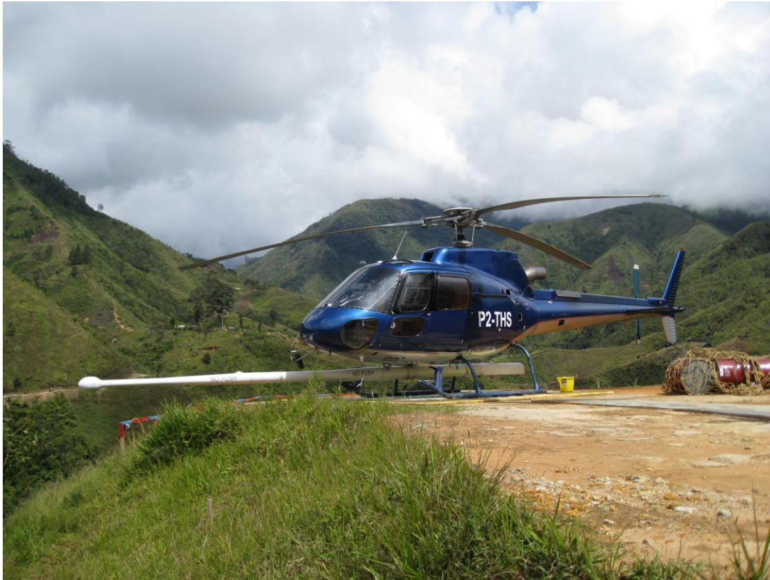
Photo of Helicopter with stinger attached for radiometric survey
