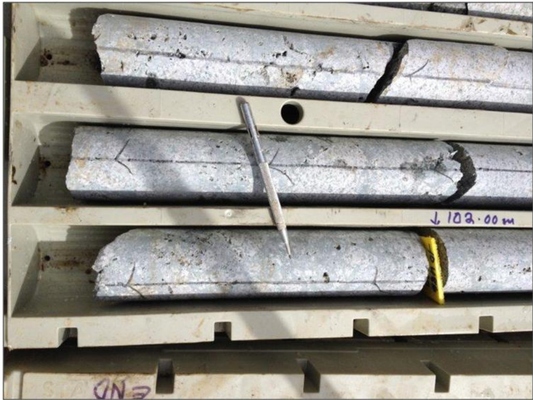
Figure 2 Oriented Core from Omora Drill Hole YD486
