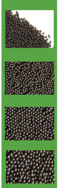
Shot (steel abrasive) is the medium used in enclosed action shotblasters, which creates the profile when impacting the surface & can be mixed & matched to improve cleaning, profiling & removal performance of the process.
