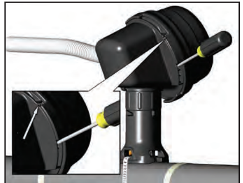
15. Lid latch mechanism fully engaged. To remove lid, repeat steps 13 and 14 but in the opposite direction.
