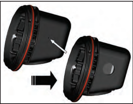
9. For power connection applications: Use dimple molded into side of junction box base to locate center of hole, drill for user supplied power connection fittings per manufacturer's recommendations.
