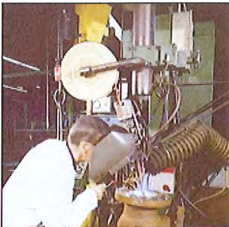
1 Automatic seal welding of Stellite 6 hardfaced seats.
