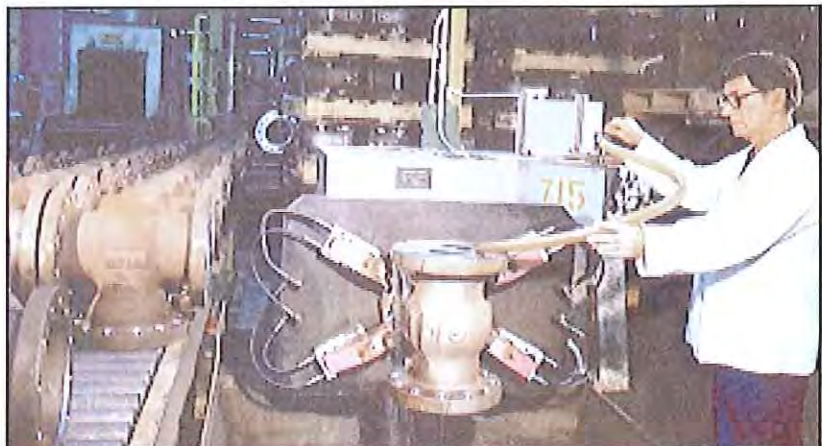
2 Air-under-water test of the seat's welds.
