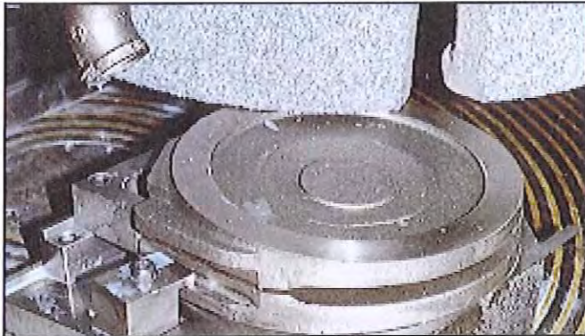
5 Precision grinding of individually fit wedge seating surfaces.
