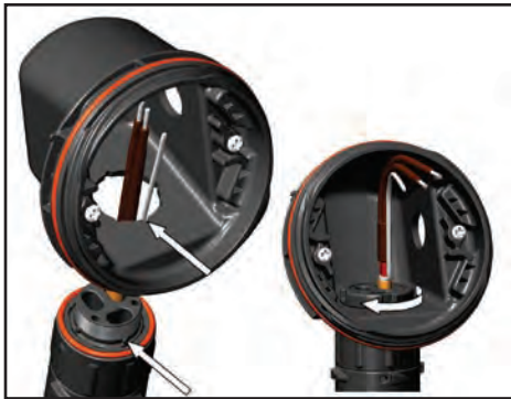
10. Mount junction box base on expediter. Make sure to align slots to properly orient junction box base. Tighten nut securely.
