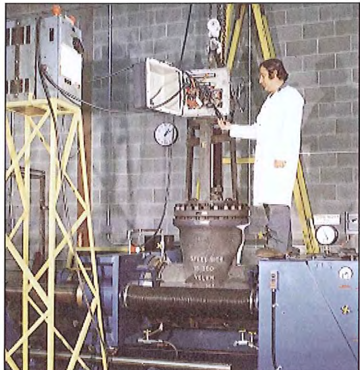
All valves are tested during production for reliability with pressurized air and hydrotested for bubble-free tightness in accordance with API 598 specifications.
