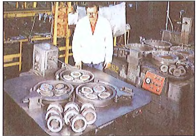
6 Lapping of wedge seating surfaces.
