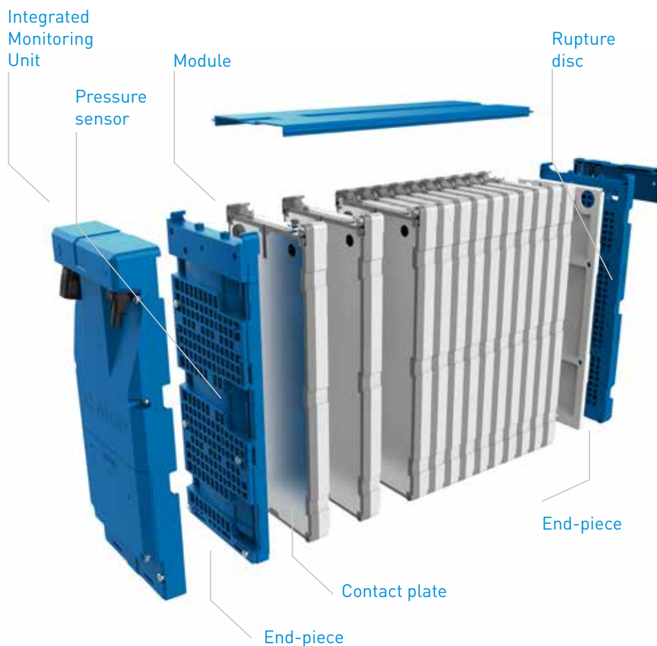
Figure 4. Battery pack expanded view.
