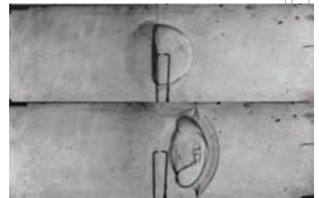
Schlieren Photography of Shock Wave Interaction with Flame Bubble
