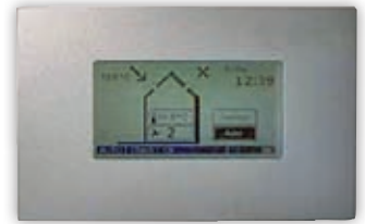
Touch screen Control panel for whole system, surface-mounting H x W x D (mm): 230 x 138 x 40
