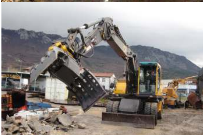
BG 13 with mounted rotator
