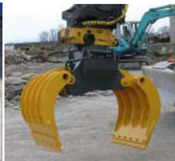
Tiltrotator enables unlimited rotation and tilting up to 40 degrees in two directions
