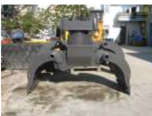
BG 13 with mounted rotator
