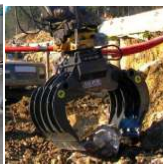
Tiltrotator enables unlimited rotation and tilting up to 40 degrees in two directions
