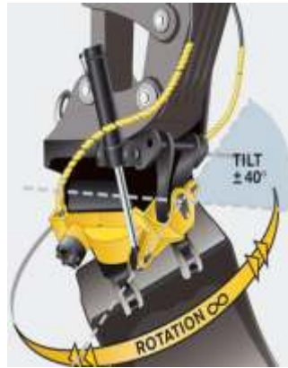
Tiltrotator enables unlimited rotation and tilting up to 40 degrees in two directions
