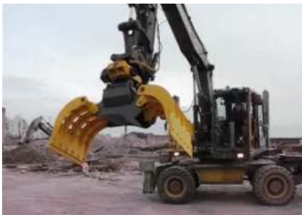
Grab BG16 on works of stone laying (making the scarps)
