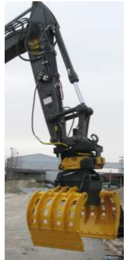
Tiltrotator enables unlimited rotation and tilting up to 40 degrees in two directions
