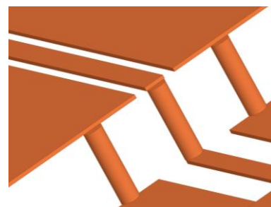
Fig. 7. Schematic view of a TSV transition from CPW transmission line on the top side of the wafer to the CPW transmission line on the bottom side.
