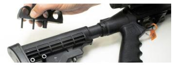
3. Put the longer screws through the rear mounting holes, the unthreaded hex standoffs and the buttstock's sling slot to screw them into the steel mounting cleat. Push the assembly as far forward as possible be-
