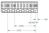
The mounting screws for the Benelli M1, Benelli M2 Tactical and Benelli M4 SureShell carriers with rails are patterned on the factory screws for the Benelli M4's optics rail. These use an unusual #8-40 thread. The above diagram illustrates the hole pattern for the SureShell carrier and rail for the Benelli M2 Tactical (dimensions in inches):
