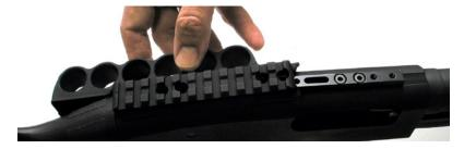
Mount the shell carrier and rail assembly to the cleat using the four shorter screws. Tighten all eight screws to about 15 inch-lbs and use a drop of blue Loctite\* on each screw.
