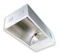
IP20 low-bay HID fitting for industrial use. Robust Steel construction with powder coated white folded sheet steel. Aluminium reflector.
