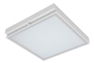
Recessed Dust Proof IP54 T5 Range designed for exposed T-Grid ceilings. The aluminium frame contains and impact resistant polycarbonate panel available in 3 options, retained by 4 wishbone springs sealing against a fitted gasket.
