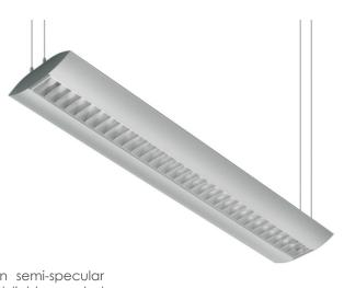
Suspended direct-indirect luminaire. Fitted with a Satin semi-specular aluminium louvre which produces controlled downward light, coupled with the upward light via a transparent perspex sheet. Manufactured from extruded aluminium and finished in Brushed aluminium. Supplied with either 2 or 4 wire suspension kits to be specified on ordering.
