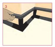
Install Capping or Diminishing Strip overlapping the Floormitres at the external and internal points.
