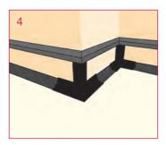
Prepared Floormitres are ready for the installation of vinyl.
