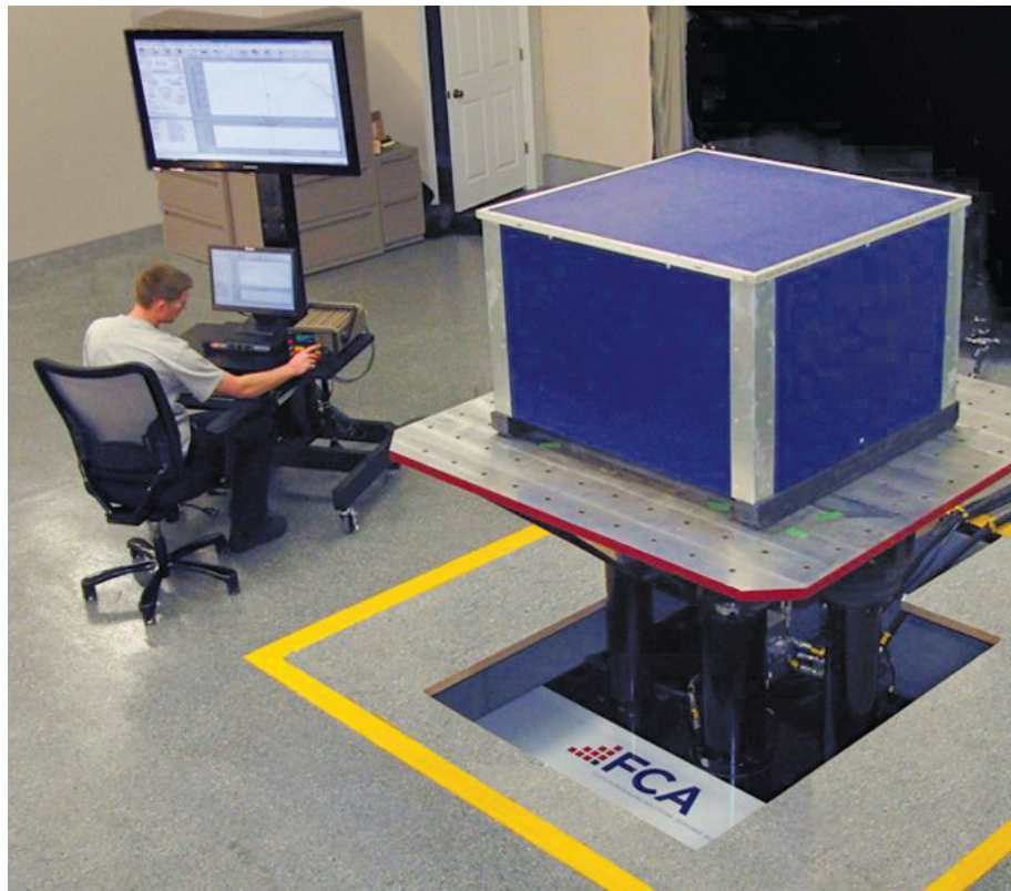
In the DTEC lab, an FCA packaging technician runs a vibration testing sequence on a custom box.
