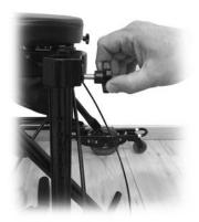
5) Loosen **Height Adjustment Knobs** so uprights can be installed. (*Left*)
