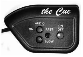
off period from 4 to 28 minutes in increments of 4 minutes; each click that sounds after pressing the button indicates 4 minutes of operating time in effect (from 1 to 7 clicks). Pressing the lower button lowers the click volume in steps to the softest setting, then recycling to the loudest setting.
