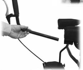
10) Install left and right handle bars and tighten bolts below the platform to secure them.
