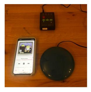
The Quick Media mode on the APPlicator quickly converts a switch press into a play/pause, skip forward, skip backward, or play for 10 seconds command.
