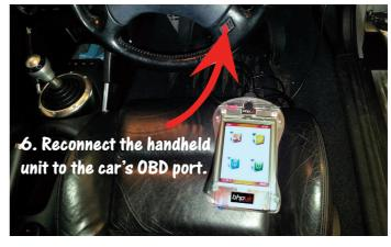
ith ease of use and convenience in mind, BHP's ECU programmer has been designed to read and program vehicle ECUs through the car's diagnostic port – meaning 99% of the time there is no need to dismantle the ECU or remove it from the car.
