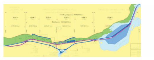
The New Suez Canal project is 72 km long and includes 35 km of the dry excavation works, with an estimated volume of  $258,000,000 \text{ m}^3$ , and 37 km of dredging and deepening works, with an estimated volume of  $242,000,000 \text{ m}^3$ .
