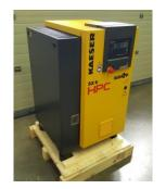
Model: HPC SX6 Rotary screw air compressor
