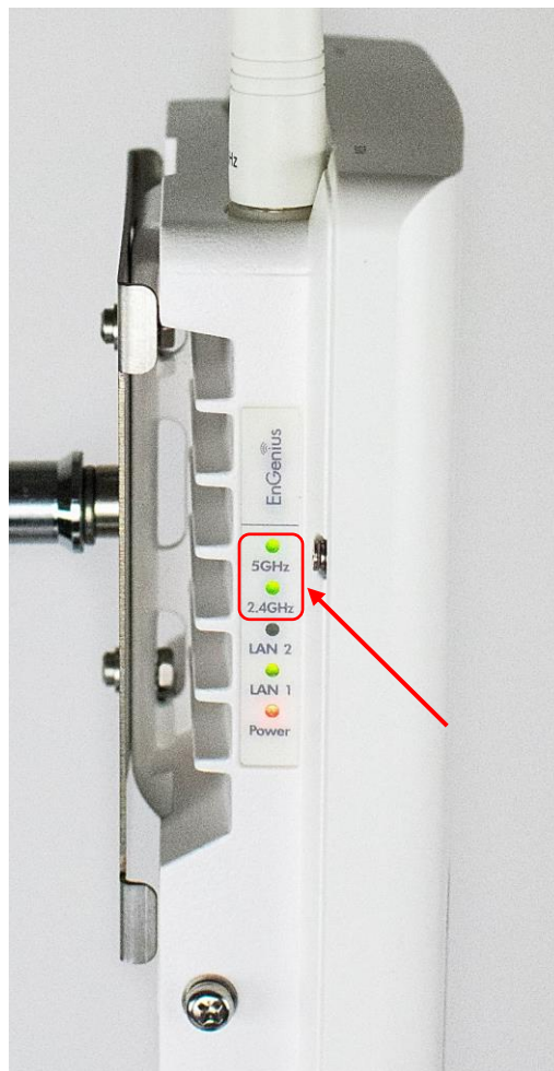
Figure 17: AP Communication LEDs
