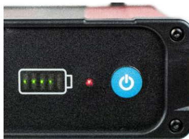
Figure 3: Power Button and Battery Status Indicator
