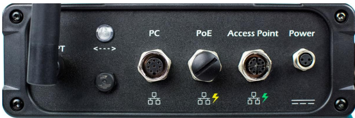
Figure 19: LAN Port Connections
