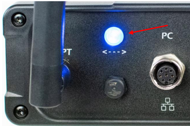
Figure 18: PC Connection Status LED
