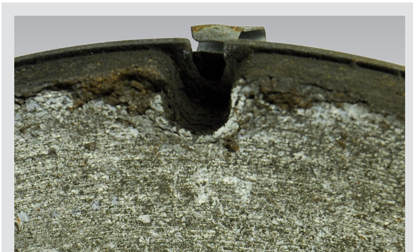
► Break-offs on the surface, no sign of high thermal stress visible
