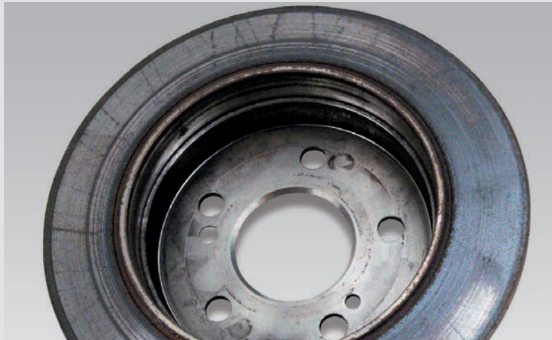
► Brake disc with static spots
