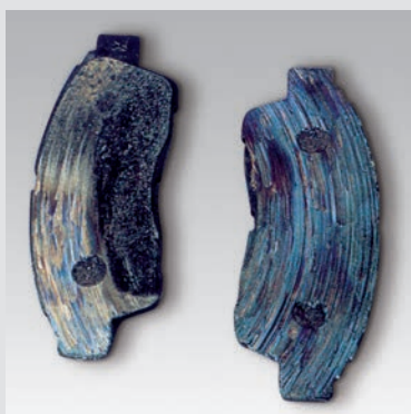
▶ Friction material worn down to the steel back plate
