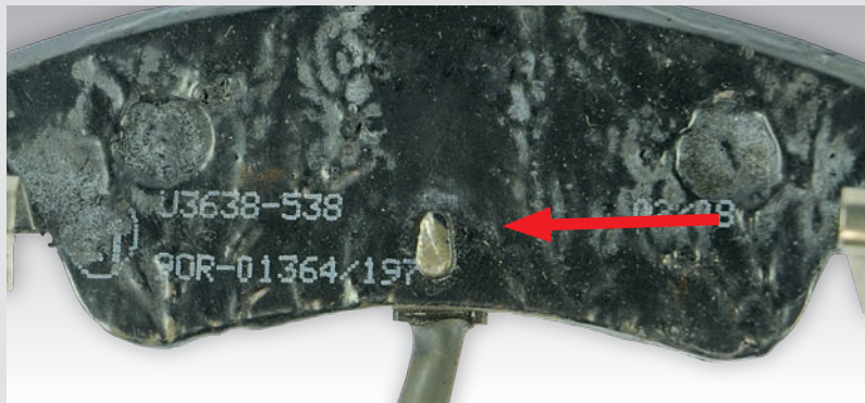
► Piston imprint on the positioning device
