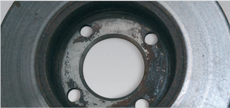
► Heavy underlying corrosion
