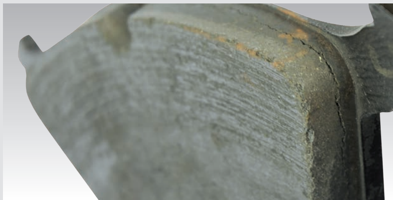
► Pad with inadmissible deterioration
