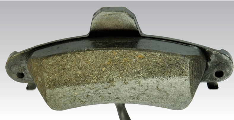
► Pad with inadequate contact pattern
