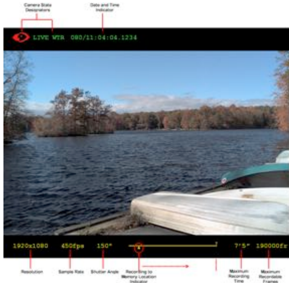
LIVE WTR Display - Recording, Waiting for Trigger Mode with an attached Phantom CineMag
