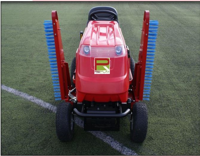
DRAG BRUSHES FOLD-UP FOR EASY TRANSPORTATION AND ACCESS
