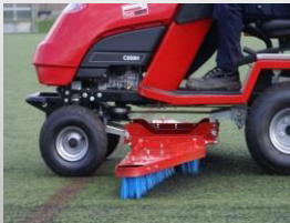
DRAG BRUSHES FOLD-UP FOR EASY TRANSPORTATION AND ACCESS
