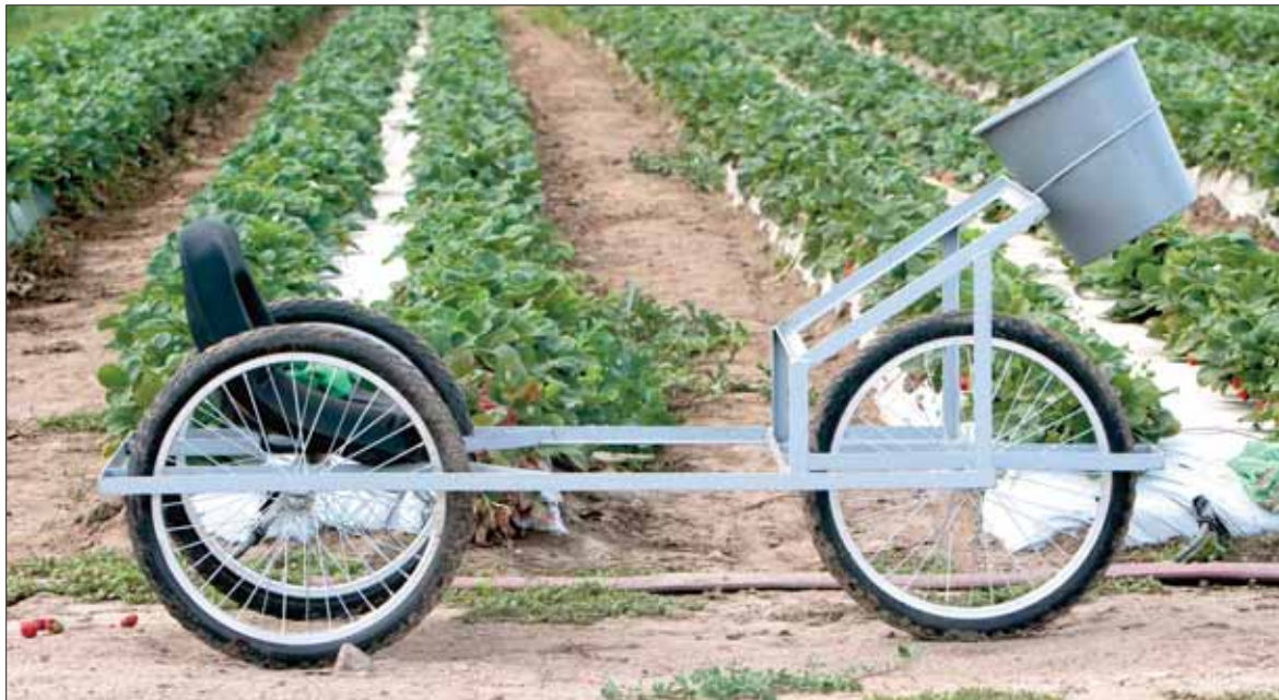
A strawberry picking cart eliminates the stress of bending over to pick fruit from plasticulture-grown berries. Photo by Glenn Lowson.
