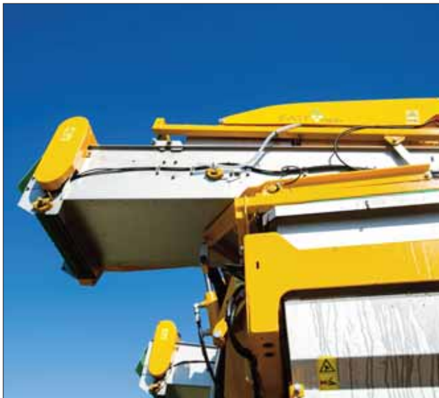
The EASYclean on-board sorting system is responsible for 99.8 per cent clean grapes without stems and petioles.
