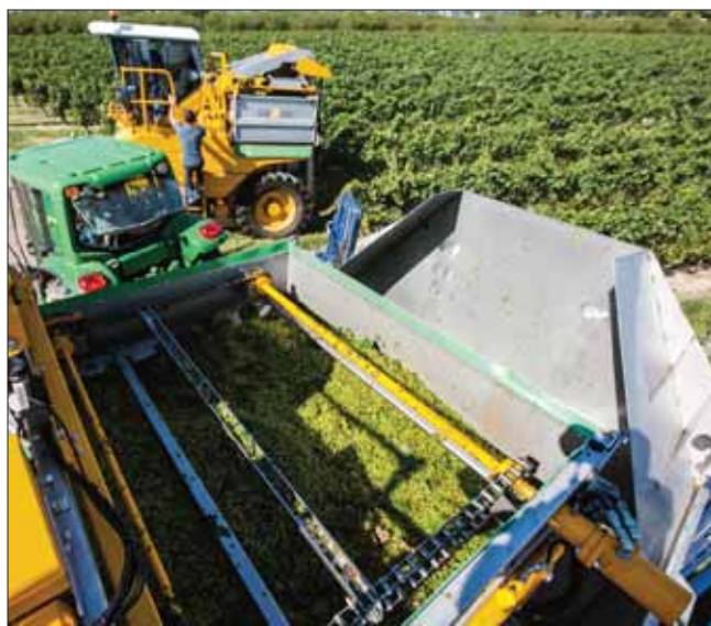
The bin capacity can hold up to 4000 liters of grapes with a tipping point of three meters.
