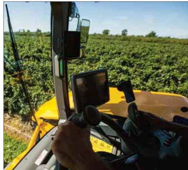
The spacious cab is equipped with a 12-inch touch screen and a multifunction joystick.
