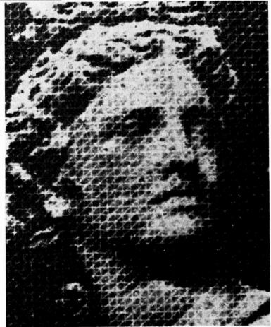
Fig. 13. Enlarged detail (10x) of Ta/bat photogravure screen (ca. 1852) incorporating a double "working-type" screen.
