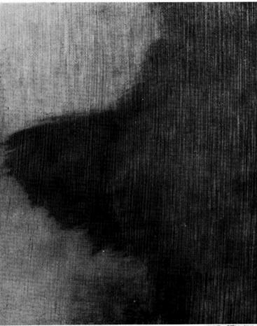
Fig. 8. Enlarged detail (10x) of a Talbot screen, a transparent, flexible sheet of cartilagionus-like material containing nearly parallel, short lines scored into both sides of sheet. Ink has been rubbed into a small area to illustrate appearance of opaque **lines**.
