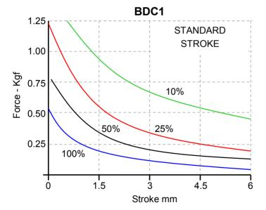
Forces shown are at working temperature Cold forces are higher
