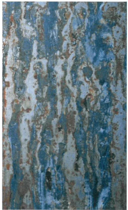
Photo 18 – G90 steel after 600h-Salt spray test, surfaces lightly brushed with water
