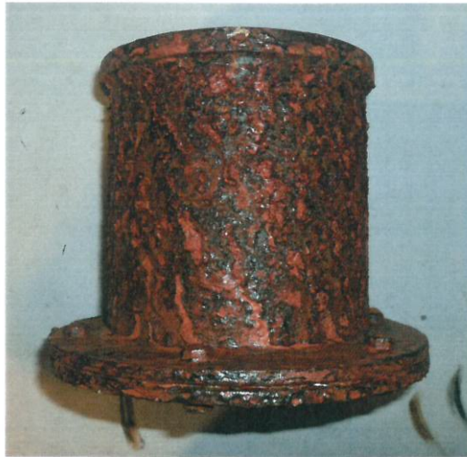
Photo 17 – RC 611 steel after 600h-Salt spray test, surfaces lightly brushed with water
