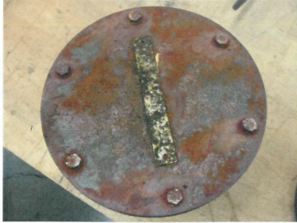
Photo 19 – RC 611 steel after 1200-Hour Moist Carbon Dioxide-Sulfur Dioxide-Air Test
