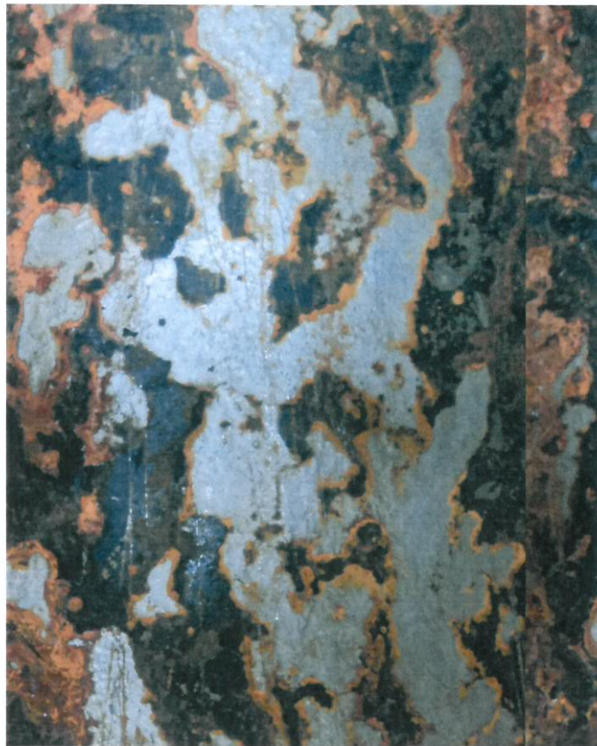
Photo 17 – RC 611 steel after 600h-Salt spray test, surfaces lightly brushed with water
