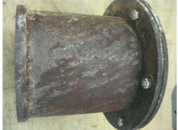
Photo 20 – RC 611 steel after 1200-Hour Moist Carbon Dioxide-Sulfur Dioxide-Air Test
