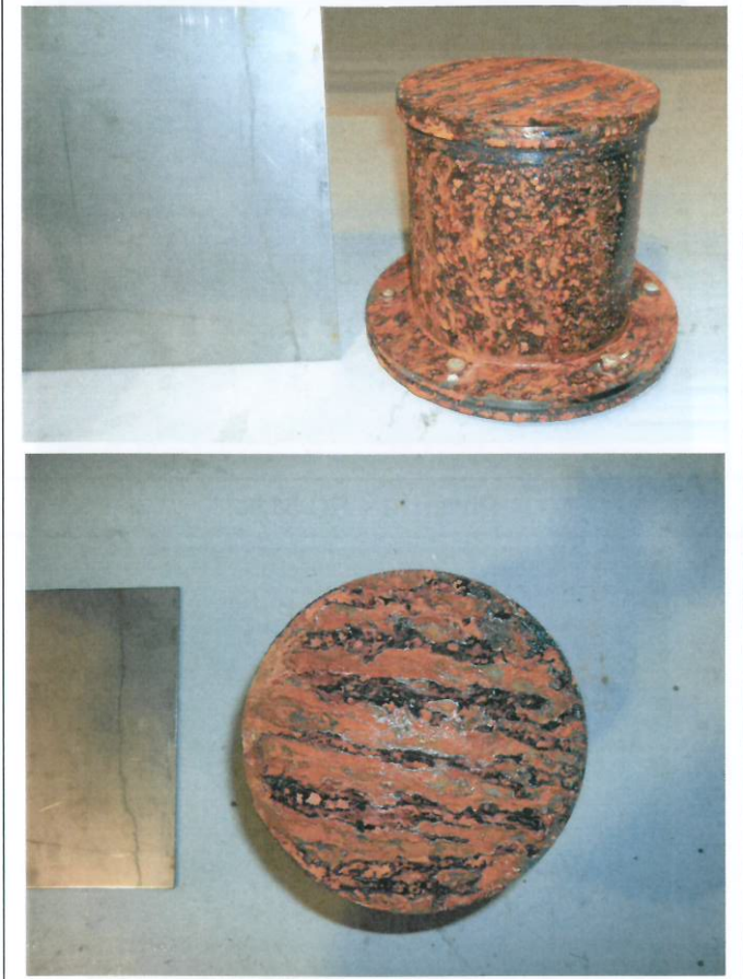
Photo 13 – RC 611 and A304 stainless steel immediately after 200h-Salt spray test
