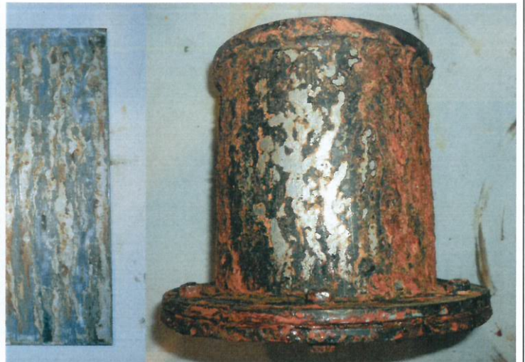
Photo 18 – G90 steel after 600h-Salt spray test, surfaces lightly brushed with water
