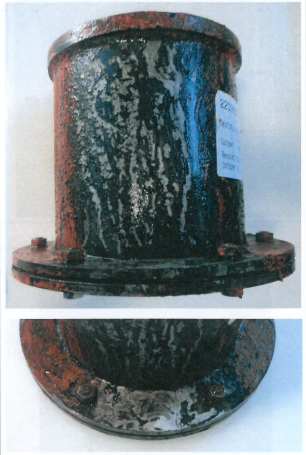
Photo 14 – RC 611 after 200h-Salt spray test, surface lightly brushed with water
