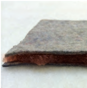
After activation, oil is solidified.
