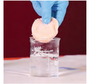
Green Rhino® CG1 Polymer is added. The spill is solidified.
