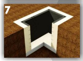
A cover frame can be fixed to chamber, once the concrete has hardened the bracing can be removed and the cover can be installed in the frame.
