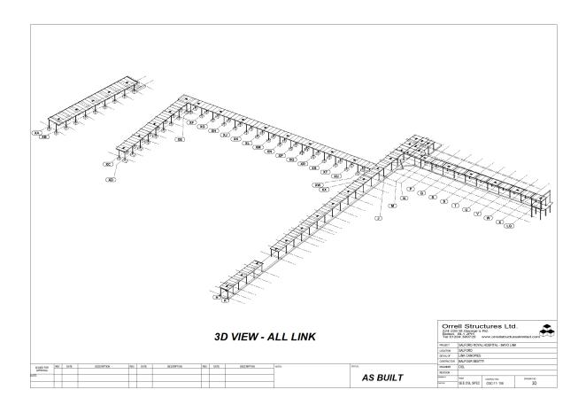
Metalwork project value £360K, mild steel painted walkway canopy incorporating green roof and mansafe system.
