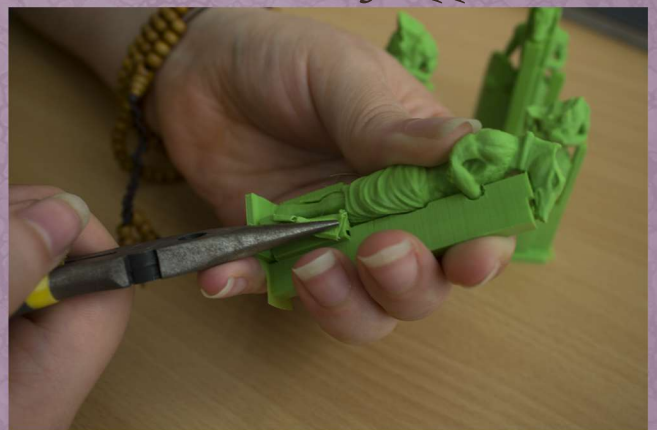
Continue breaking supports
