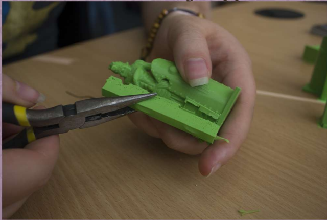
Continue breaking supports
