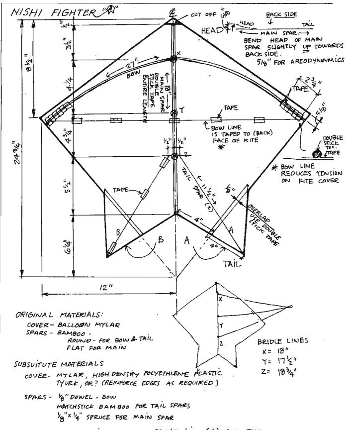
NOTE: FOLD MATERIAL ALONG CENTER LINE (4) AND THEN CUT THIS INSURES SYMMETRY !!
