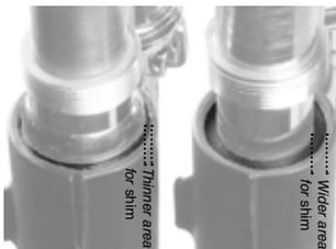
Notice that the slide on the left requires a very thin shim while the slide on the right requires a thicker shim.
