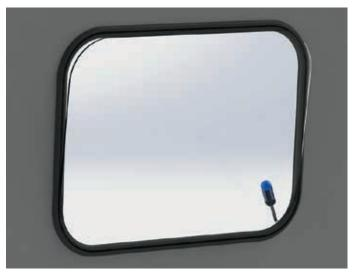
Next pour a small amount of diluted washing up liquid in the glass groove of the window rubber to make it easier to fit. Now take the glass and insert it into the bottom groove of the window rubber. Using the glazing tool you can lever the glass into the window rubber groove all the way around.
