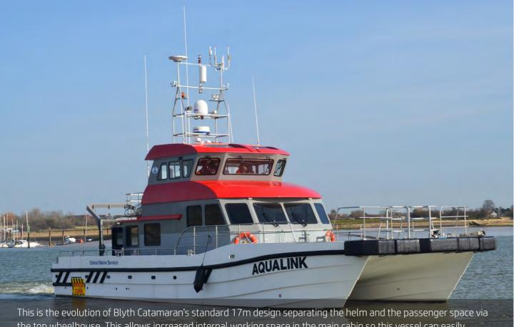
the top wheelhouse. This allows increased internal working space in the main cabin so this vessel can easily accommodate both survey duties and also crew transfer duties both to ships and windfarm turbines.
