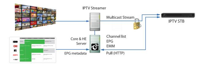
The Channel list, EPG and EMMs for decryption can either be pulled from an URL address by the STBs or sent to the STBs in a separate Multicast Stream from the IPTV Streamer. This way of providing the streams is more affordable and scales better than systems where a middleware server from a third-party provider is used.
