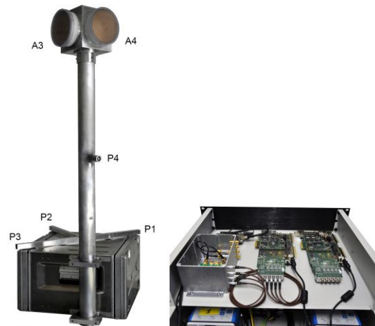
Fig. 3. Left: prototype of the PROGRESS PADS electronics box with mounted pressure sensors ( P_n ) and antennas ( A_n ). Right: view into the 19-inch drawers.
