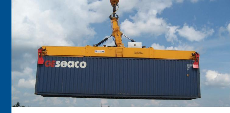
The RAM 2700 series of Electro-Hydraulic Telescopic Spreaders including twinlift has been developed to provide productive, safe and cost-effective container handling for mobile harbour and jib cranes. Six models provide a wide choice of capacities from 35 to 60 tonnes designed to handle single 20', 40' and 45' containers. 2740, 2750 and 2760 models also provide twinlift capability, designed to handle two 20' containers as well as the full range of single container lifts.
