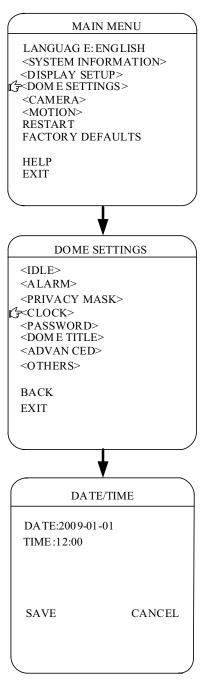
The clock is used to program the current date and time. The date and time set in the Clock menu is used to program events. The date and time can also be displayed on the monitor when the menus are not being accessed.
