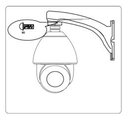
(4) Use screw-caps and shims to fix the bracket on the wall.
