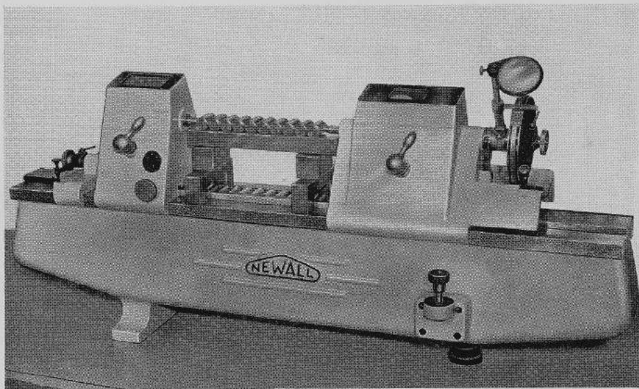
A Newall Linear Measuring Machine employed in checking 10 rollers, of the Newall patented measuring system, against 10 master rollers calibrated by the National Physical Laboratory.
